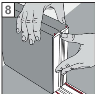
8. While glueing the profile to the glass block vertically make sure it touches the long floor profile. The short profile shouldn't protrude the glass block as this may cause alignment issues later on.
