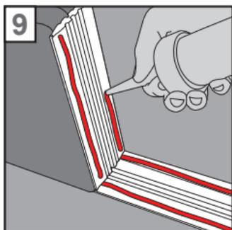
9. Apply adhesive to the short profile you just glued to the glass block and sprinkle the adhesive with water.
