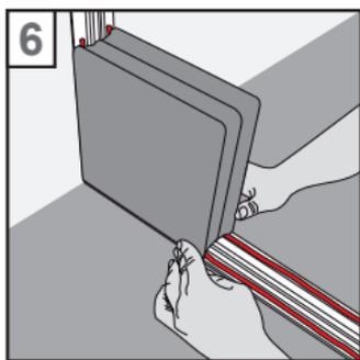
6. Now place the first glass block onto the profiles. Positioned correctly, the glass block should descend a little. Make sure the adhesive attaches properly, by lifting the glass block very cautiously.
