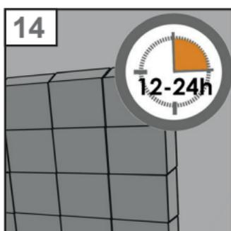
14. We recommend waiting 12-24 hours after installing about 4-5 rows in order to let the adhesive dry. Doing so will help you avoid any deformation caused by the glass blocks' weight. In any case, wait at least 24 hours before jointing the finished wall.
