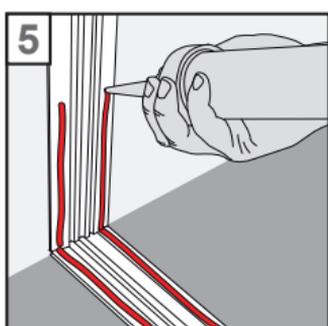
5. Apply adhesive to the wall profile, up to the height of one glass block. Sprinkle the glue with water.
