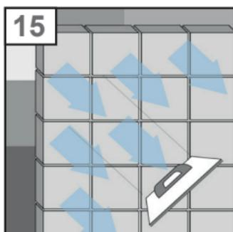
15. To joint the wall, use our glass block joint grout FlexFluge. Use a spline or rubber spatula and apply the joint compound diagonally. Fill in the joints completely and smoothen them with a wet sponge afterwards. Remove the remaining joint compound from the glass blocks.
