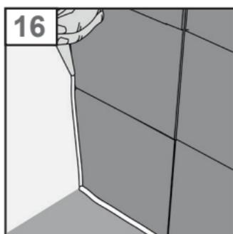
16. Finally, use an appropriate silicone for sealing the connection joints to the wall and ground. **Do not** use SRT adhesive for this step!
