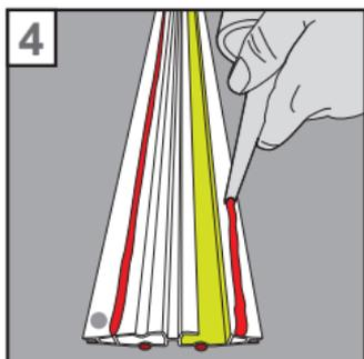
4. Now apply construction adhesive to the smooth surface of the profile and sprinkle it with water. CAUTION: Work neatly, as any adhesive getting into the CHANNEL may block the LED stripe from being installed correctly.
