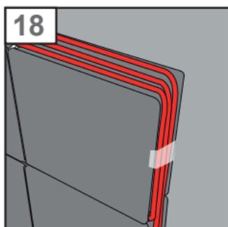
18. Place the LED stripe cables neatly against the recess of the glass block. Fix the cables with tape if necessary. To ensure that the end profiles can be attached to the wall without any problems, no cables must protrude from the glass blocks.
