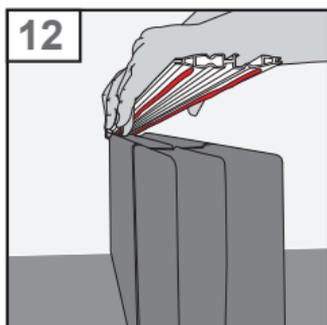
12. Now take a profile with a CHANNEL (marked with a label); the CHANNEL faces upwards. Apply adhesive to the middle of the smooth surfaces. Afterwards, position the profile, with the adhesive facing down, on your glass block row. Gently press onto the profile to make sure the adhesive sticks to the glass blocks properly.
