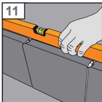
11. Once the first row is done, use a spirit level to check if all glass blocks are straight in line. As long as the adhesive SRT hasn't hardened, you can make slight adjustments.
