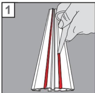
1. Ground profile installation: Take a profile with a CHANNEL (marked with a label); the CHANNEL faces downwards. Apply about 5-6 mm of mounting adhesive to the profile's recesses and sprinkle it with water.
