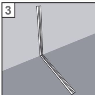
3. Wall profile installation: Take a profile without CHANNEL (no label marking) and attach it just as you did with the ground profile. Afterwards, make sure the angle between both profiles is 90°.
