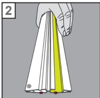
2. Decide which direction you want the LED lights to shine in and place the CHANNEL accordingly. All other rows will be positioned the same (see step 13 on page 16). Now turn the profile around so the side the adhesive was applied to faces down, and firmly press the profile to the ground. The CHANNEL now faces upwards.
